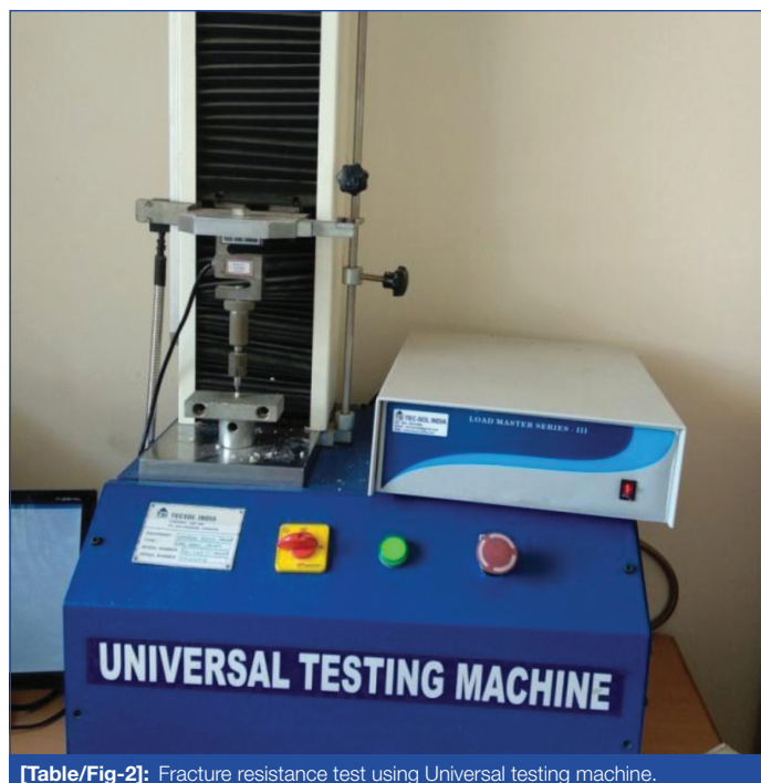
[Table/Fig-2]: Fracture resistance test using Universal testing machine.
